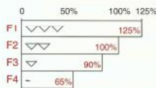
Chart of difference in holding power by attractive face roughness For all models
